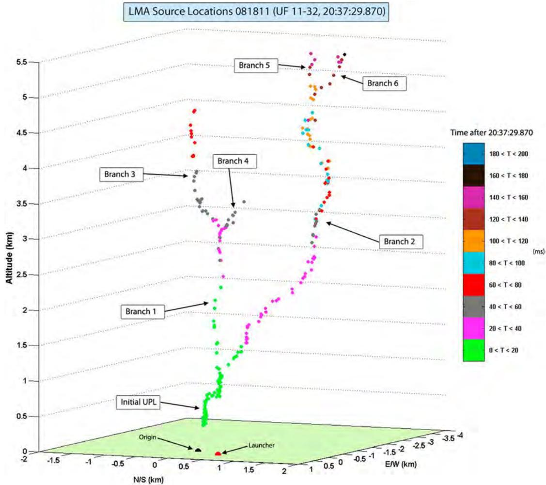
**Figure 2.** Three-dimensional view of the LMA source locations associated with the sustained UPL/ICC of flash UF 11-32 on August 18, 2011. Sources correlated in time with precursor current pulses and diffuse sources not obviously corresponding to extensions of previous branches have been removed. The sources are color coded in time according to the key at right in 20 ms time windows. The launching facility and coordinate origin are labeled.
