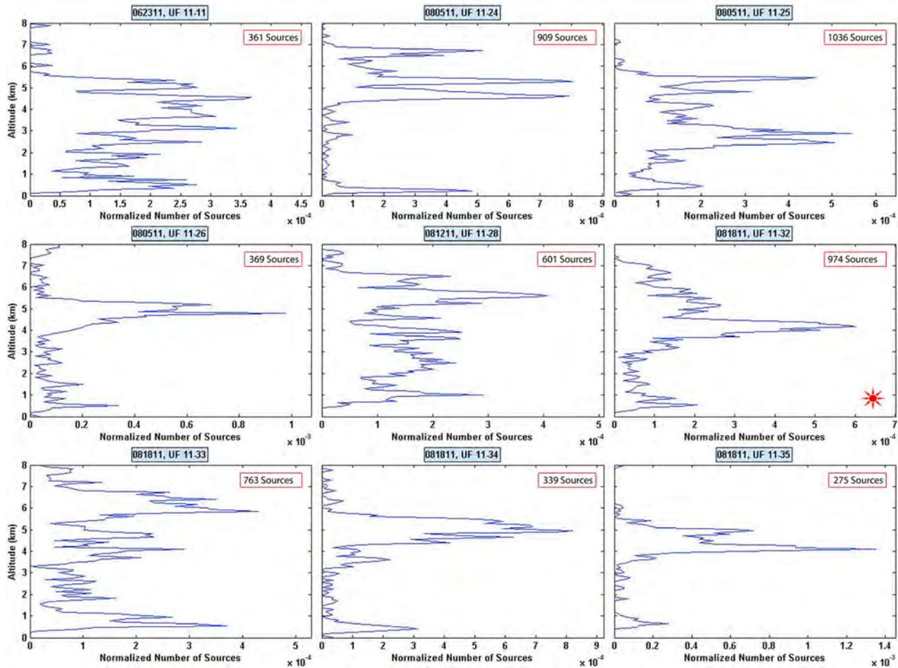
**Figure 4.** Histograms (bin size equal to 30 sources) of the altitude distributions of LMA sources for nine triggered lightning flashes. Source altitudes below 8 km are plotted. The histograms are derived from sources extending only from the time of the rocket launch through the end of the IS period. The peaks of the histograms are indicative of the altitude region where the IS transitioned from vertical to more horizontal propagation.
