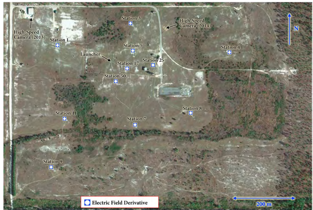
Figure 1. Aerial photograph of the ICLRT showing the locations of the dE/dt measurement stations, the high-speed camera locations, and the launching facility.
